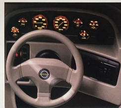
Instrumentation in the 1750 SE includes critical engine monitoring gauges as well as a tachometer, speedometer, and a trim indicator gauge.
