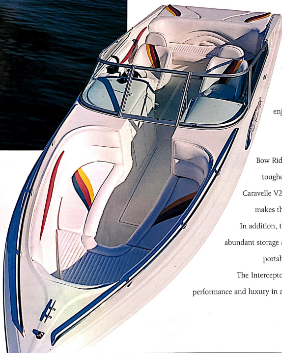
The Caravelle V24 Offshore Hull is a premium performer for big water boats, with an aggressive 24 degree deadrise that cuts through rough water for a smooth ride.
