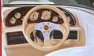
Standard helm features a digital hour meter, digital depth finder, tilt steering and a CD player.
