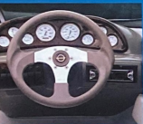
Standard helm features a digital hour meter, digital depth finder, 12 volt receptacle, tilt steering and a CD player.
