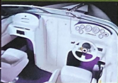
Sport dash features a digital hour meter, digital depth finder, tilt steering, 12-volt receptacle and a CD player.
